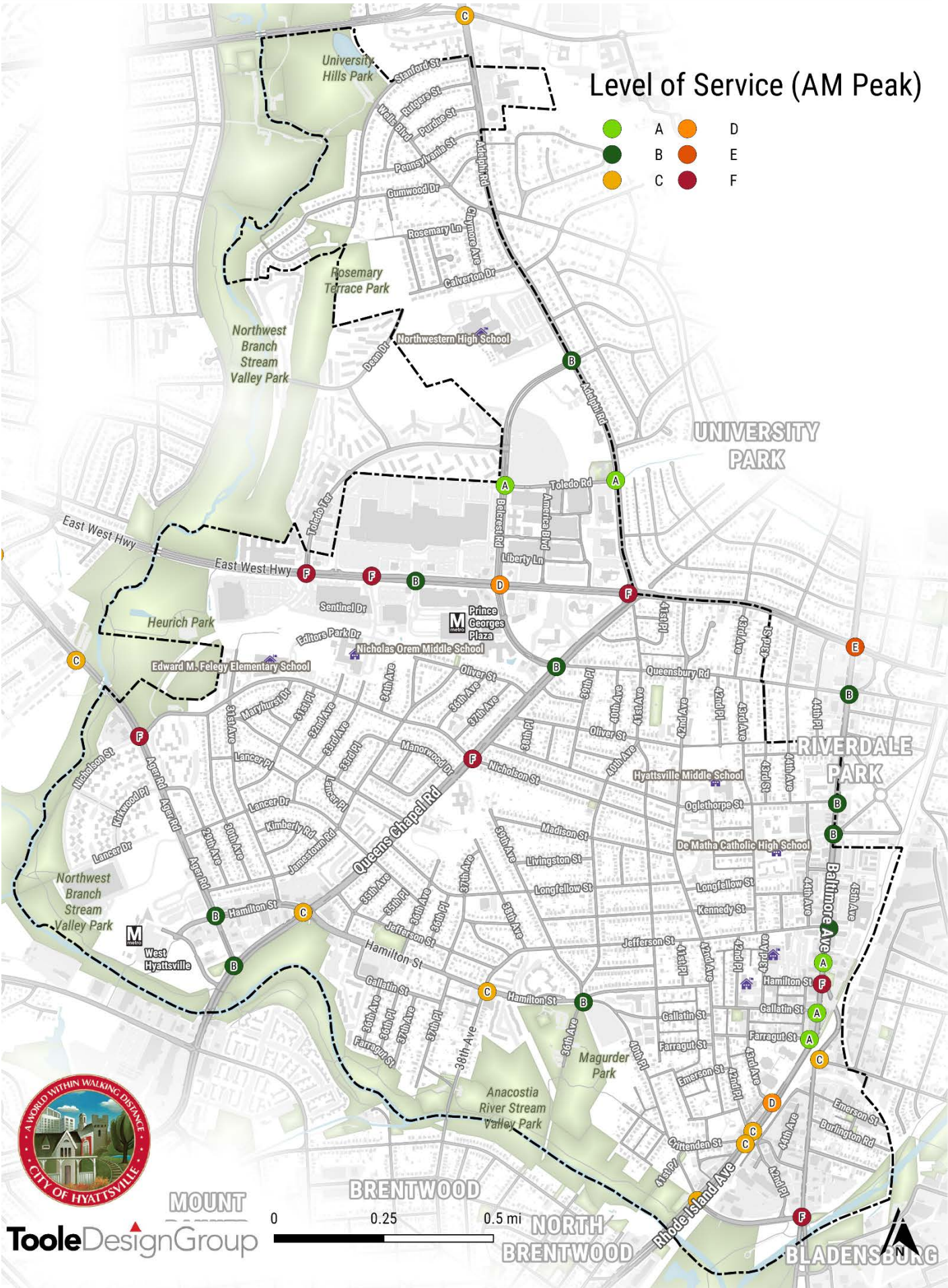
Figure 37: Level of Service (AM Peak)
