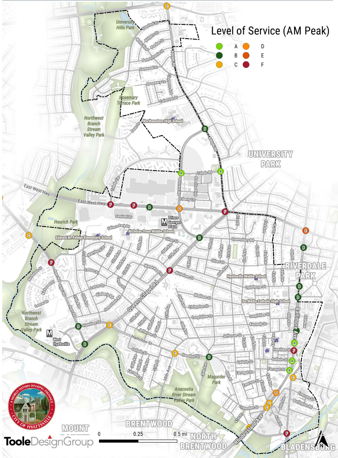
Figure 37: Level of Service (AM Peak)
