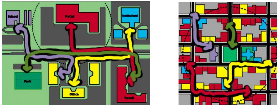
Sparse street network (left image) concentrates traffic on small number of street, while dense connected street network (right image) distributes the traffic evenly and improves resiliency.
