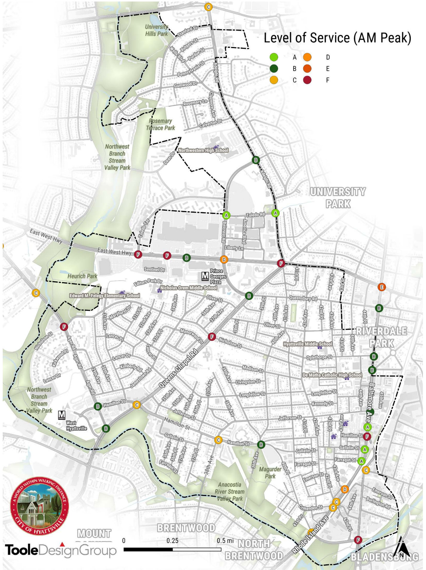
Figure 37: Level of Service (AM Peak)
