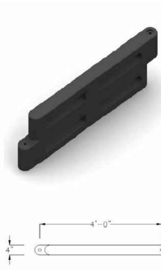
14 Poly-timber Borders or Approved equal 7 NOT TO SCALE
