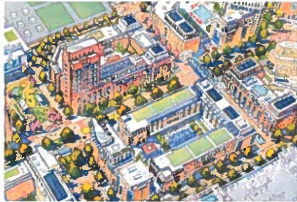
Example of an illustration of a street network design with a maximum 500 feet block configuration.
