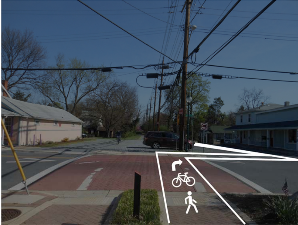
Figure 28 - Northbound view at the Berwyn Road intersection, with an illustration of potential location of pavement markings to direct users to the appropriate Trail path.
