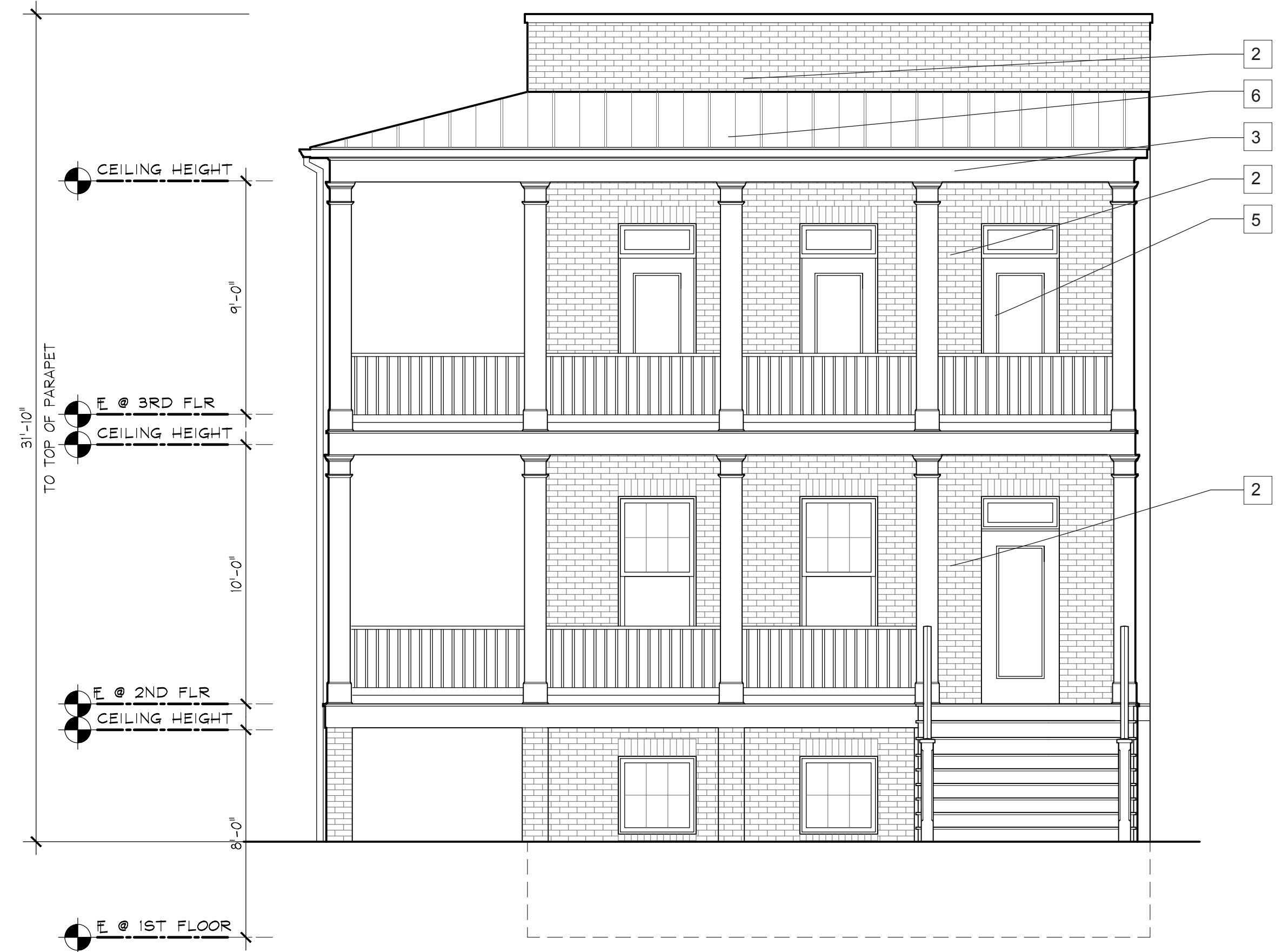
1 FRONT ELEVATION - 2-STORY PORCH A2.5 1/4" = 1'-0"
