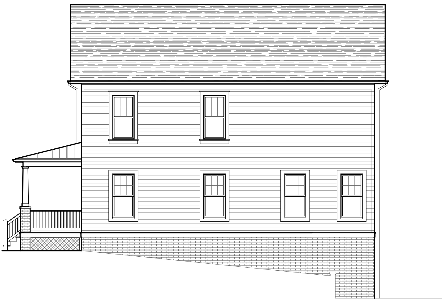
4 SIDE ELEVATION A2.2 1/8" = 1'-0"
