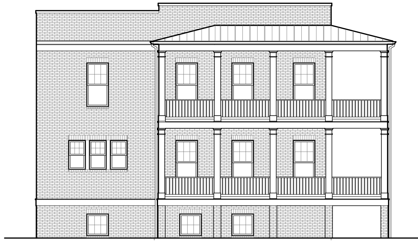
3 SIDE ELEVATION - 2-STORY PORCH A2.5 1/8" = 1'-0"
