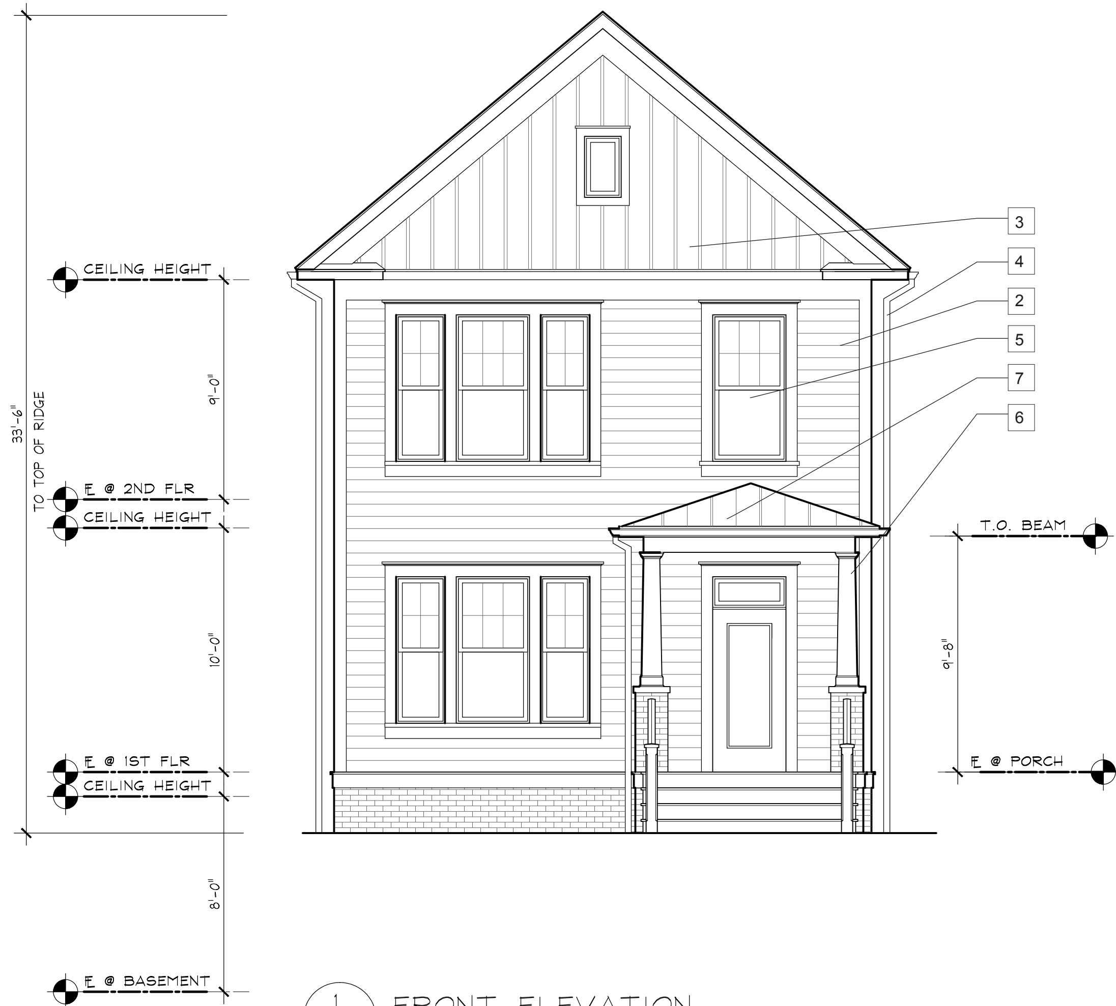
1 FRONT ELEVATION A2.2 1/4" = 1'-0"
